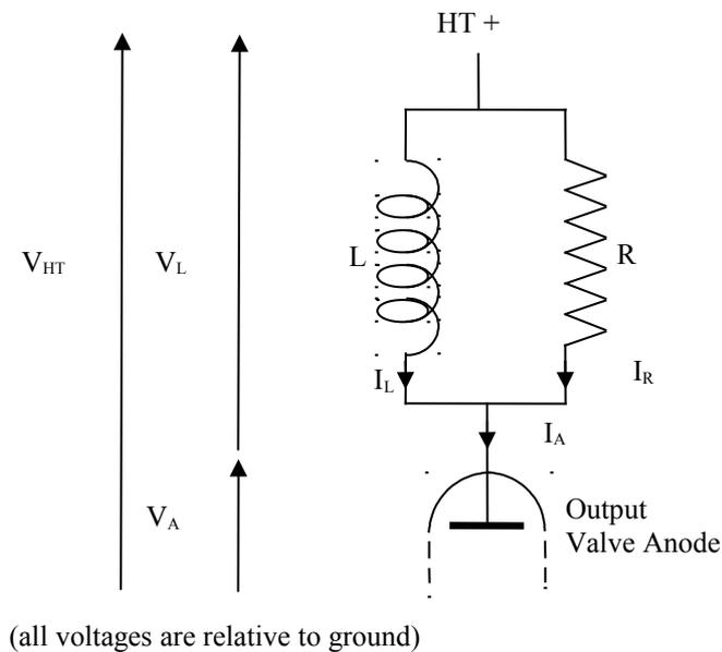
Figure 1: Approximate Equivalent Circuit Model
