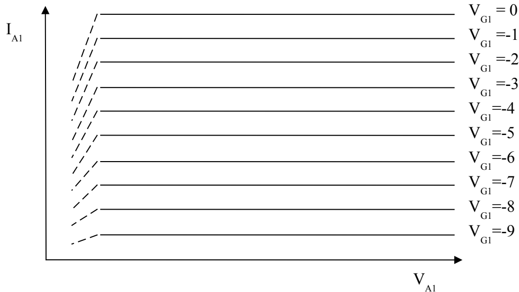
Figure 2: Ideal (Fictitious) Pentode Characteristics
